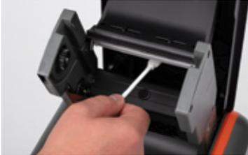
6. Run the swab or cloth between and around the gray adjustable label guides in the floor of the printer, to clear any dust or adhesive build-up.
