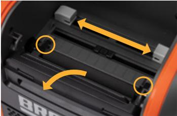
8. Finally, use the swab or cloth to clean both sides of the cutter blade, by gently inserting the swab into the slot of the cutter module and sliding it from side to side. Repeat this process for the front and the back of the blade; the cutter module can be flipped forward to make the back easier to reach.
